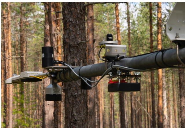
Fig. 5. Machine sensing of climate conditions at Oulanka Research Station, Finland. (© Cesar & Lois. Photo: Cesar & Lois.)
